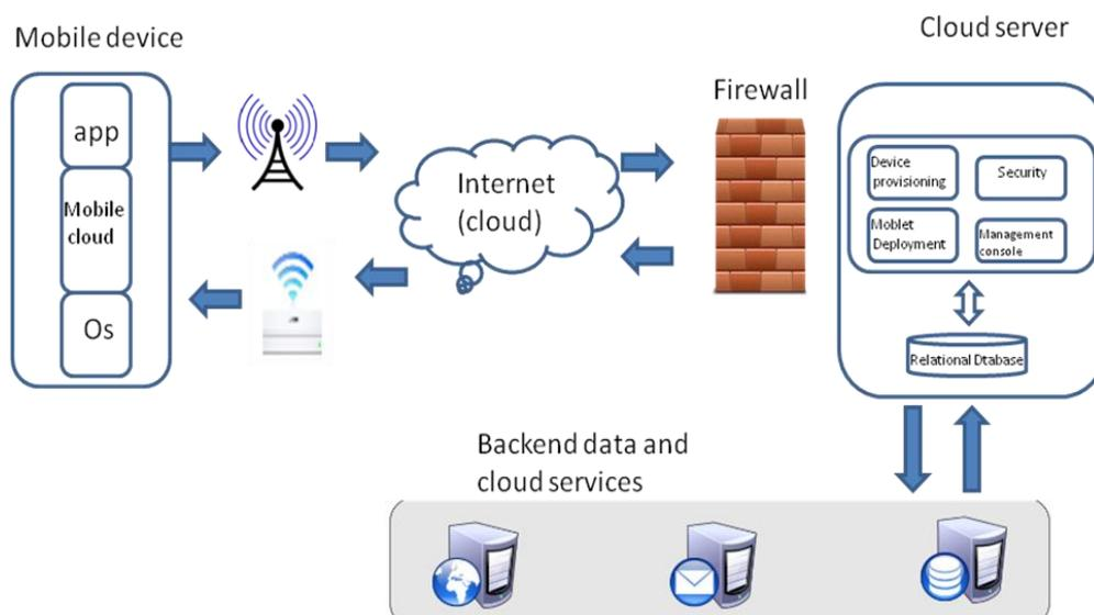
Fig. 1: Architecture of mobile cloud computing.
