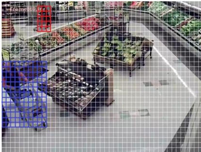
Fig.3. Result after spatial filtering tracked in consecutive frames (shows macroblock having motion)
