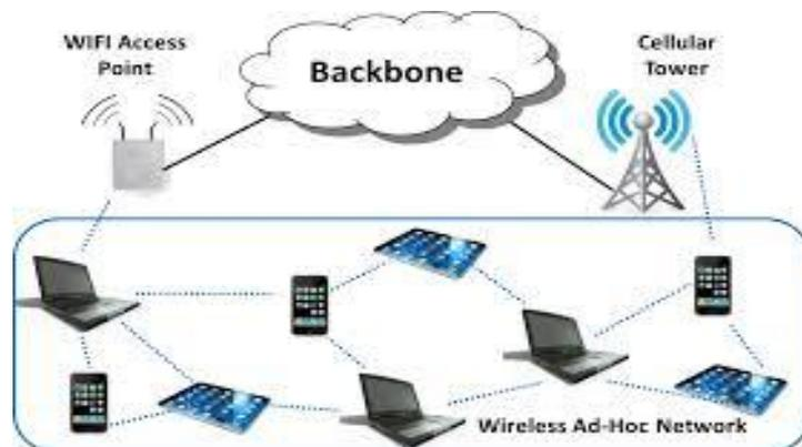
Fig 2. Wireless MANET connection
