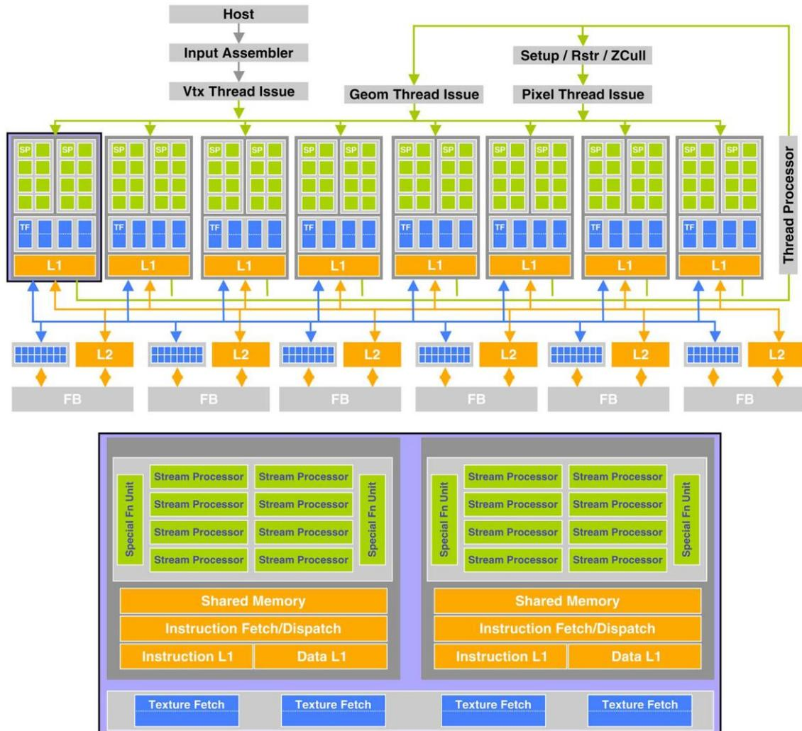
Fig. 2 NVIDIA build architectures with unified, massively parallel programmable units at their cores. The NVIDIA GeForce 8800 GTX (top) features 16 streaming multiprocessors of 8 thread (stream) processors each. One pair of streaming multiprocessors is shown below; each contains shared instruction and data caches, control logic, a 16 kB shared memory, eight stream processors, and two special function units. (Diagram courtesy of NVIDIA.)[5]
