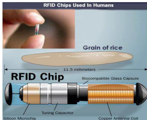
Fig 5 Verimed with Tuning Capacitor
