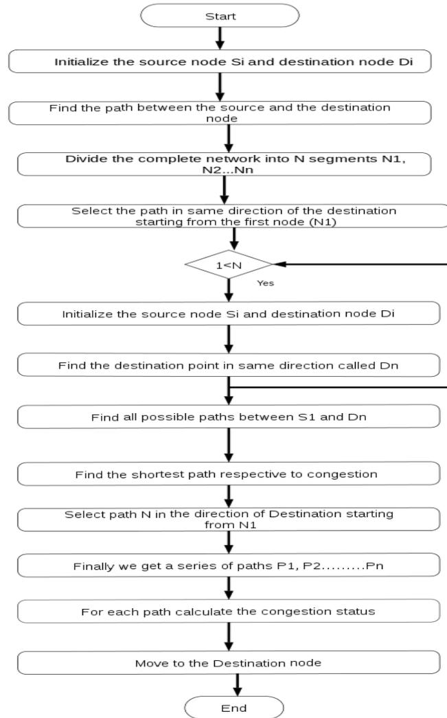
Fig. 2 Alternate road selection flow chart
