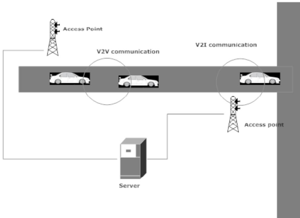
Fig. 1 Communication Architecture of VANET
