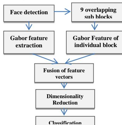
Fig. 2 FLOW DIAGRAM OF THE SYSTEM
