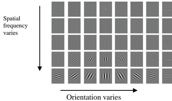
Fig. 3 REAL PART OF GABOR FUNCTION FOR FIVE DIFFERENT SCALES AND EIGHT DIFFERENT ORIENTATIONS
