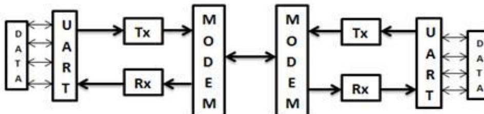
Fig. 7: Serial data transmission and reception in UART.
