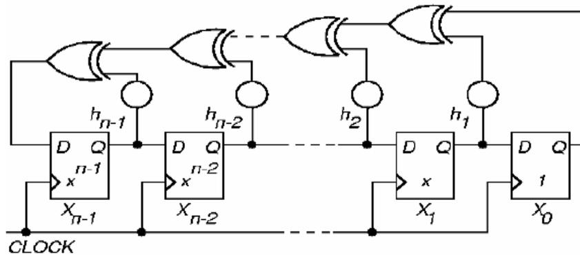
Fig. 6: Standard n-stage LFSR circuit
