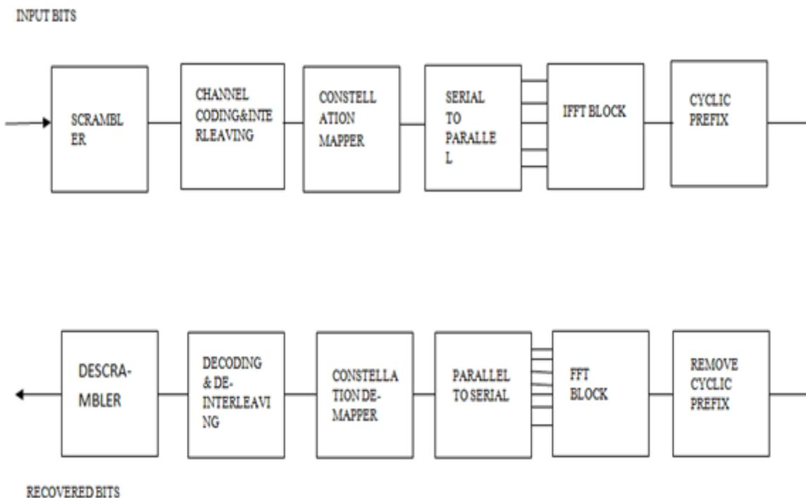
Figure 2 Transceiver for 802.11a
