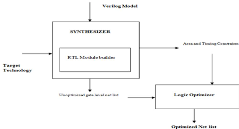
Figure 3 Synthesis Process in VERILOG
