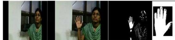
Figure 3: a) Background Image b) Foreground Image c) Subtracted Image d) Segmented Image
