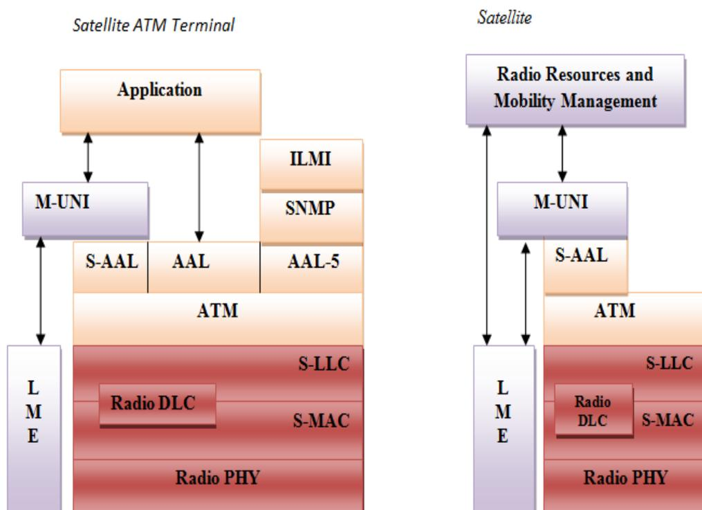
Fig. 2 ATM- Sat Protocol Stack
