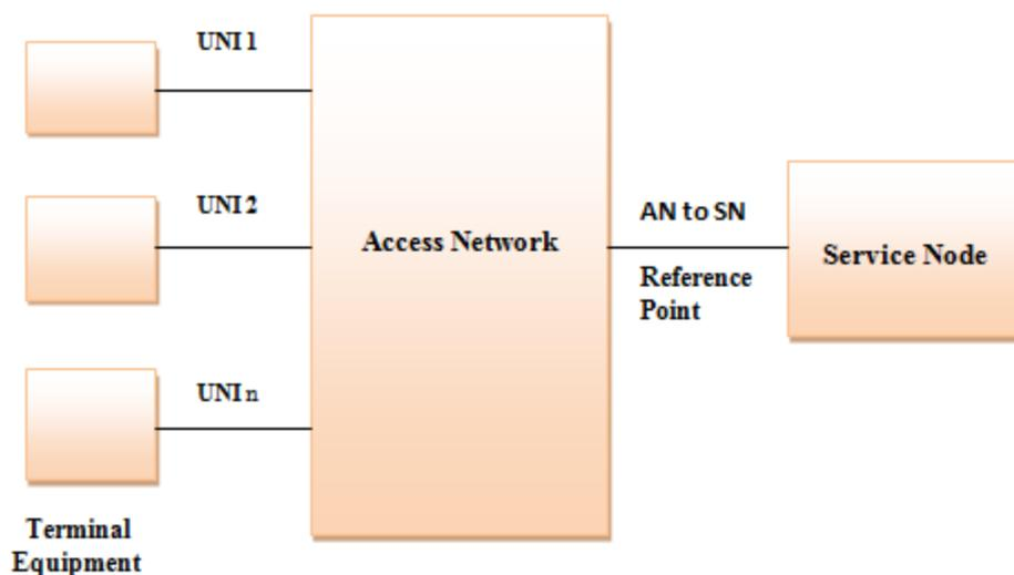
Fig. 1 Generic Broadband Access Network Configuration
