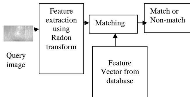
Figure.1 Block diagram of the knuckle print recognition system.
