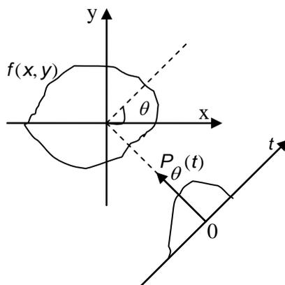
Figure.2 Radon transform  $P_{\theta}(t)$  is the 1-D projection of  $f(x, y)$  at an angle  $\theta$ .
