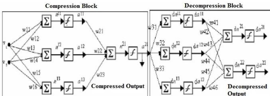
Fig1. Image Compression and Decompression using proposed neural architecture.
