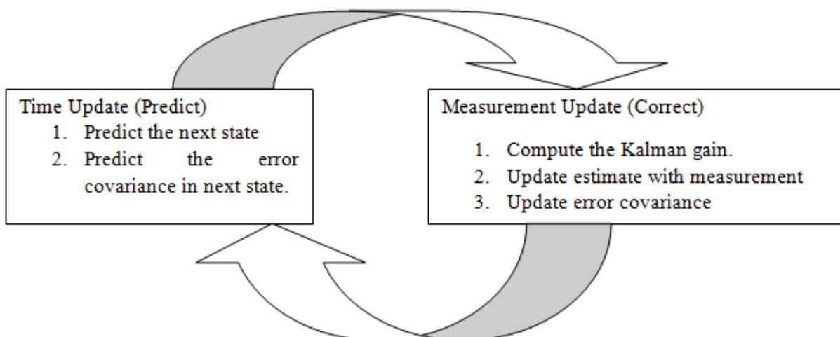
Figure 2 Working of Kalman Filter
