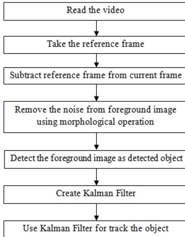
Figure 3 Flowchart of Proposed Method for Object Detection and Tracking
