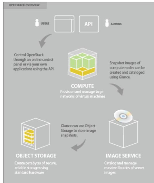
Figure 4 OpenStack Architecture
