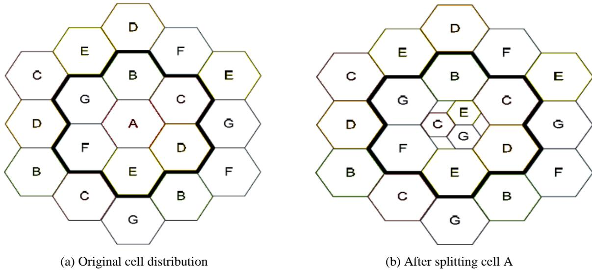
Figure 1.5: Example of cell splitting
