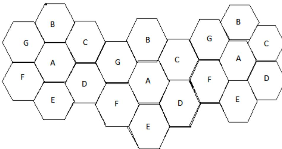
Figure 1.6: Representation of Frequency reuse concept
