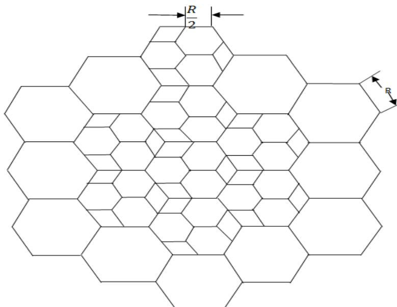
Figure 1.4: Each cell in a cluster is split into approximately four smaller cells by reducing R by half.
