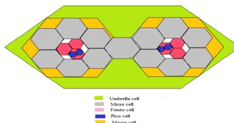
Figure 1.2: Representation of cells according to their size
