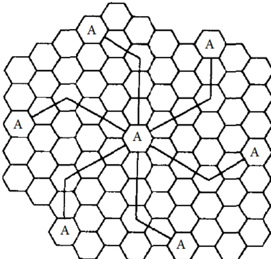
**Figure 1.8:** An example of frequency reuse with  $N = 19$  [14]
