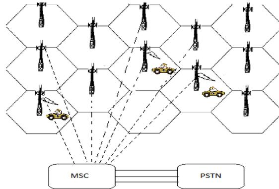
Figure 1.3: Representation of basic Cellular system [14]
