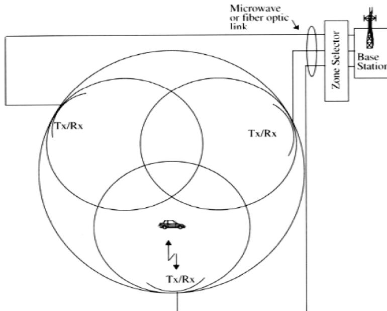
Figure 2.3: Microcell zone concept[14]
