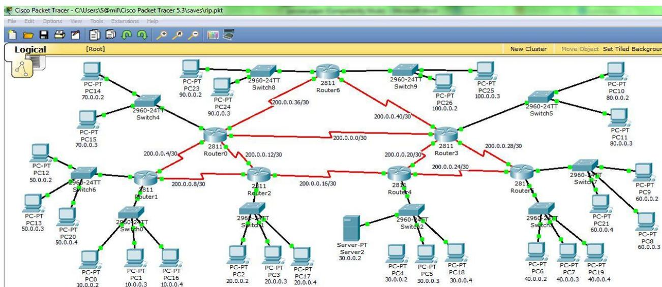
Fig. 1 A simulation of RIP in cisco packet tracer
