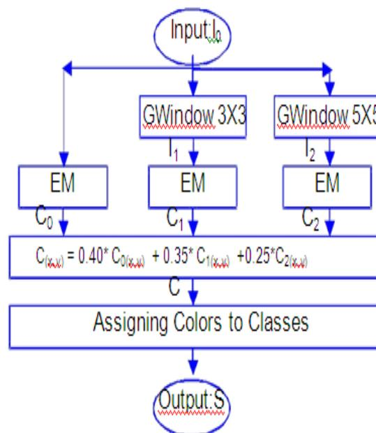
Fig: 3 The GMEM flowcharts, the input is the image to be segmented,  $I_0$  and the segmented images  $S$ .
