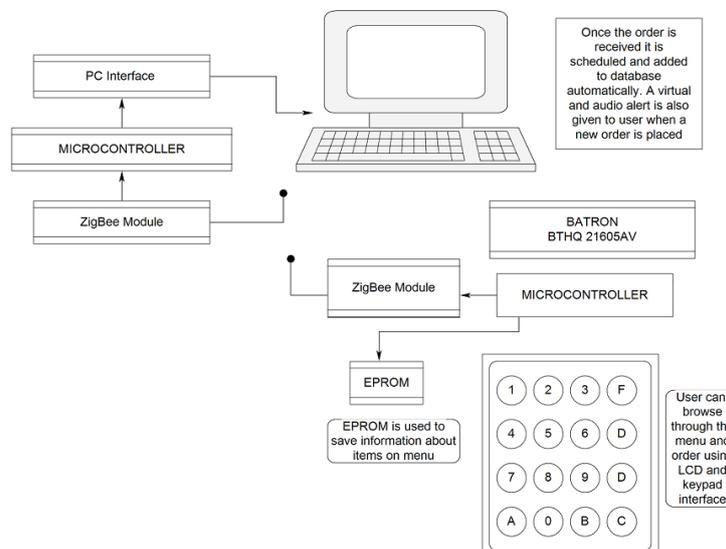
Fig. 1 Block Diagram for Transmission & Reception.
