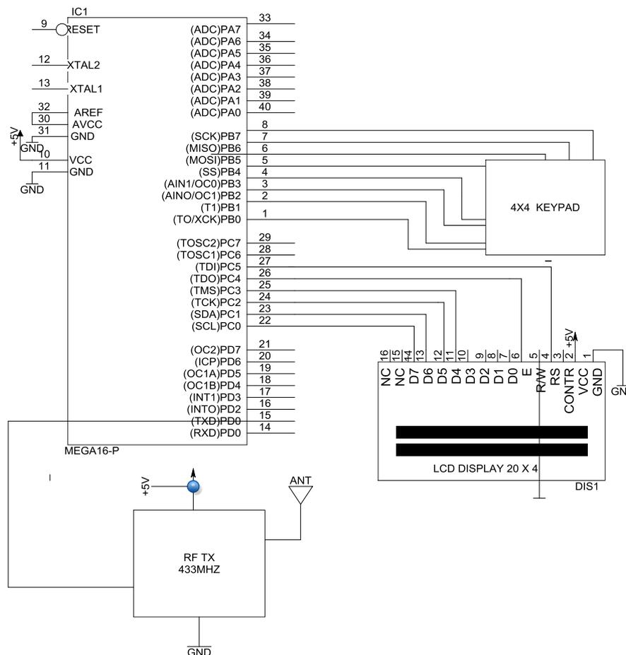
Fig. 2 Pin Diagram for Transmission and Reception.
