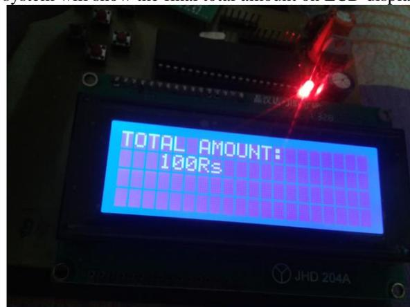
Fig. 5 LCD display showing the total amount
