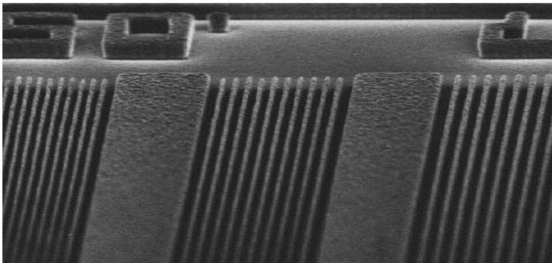
Fig-1: Using a prototype system, the Virtual National Laboratory has successfully printed lines as small as 50 nanometers (billionths of a meter) wide in photo resist[4]
