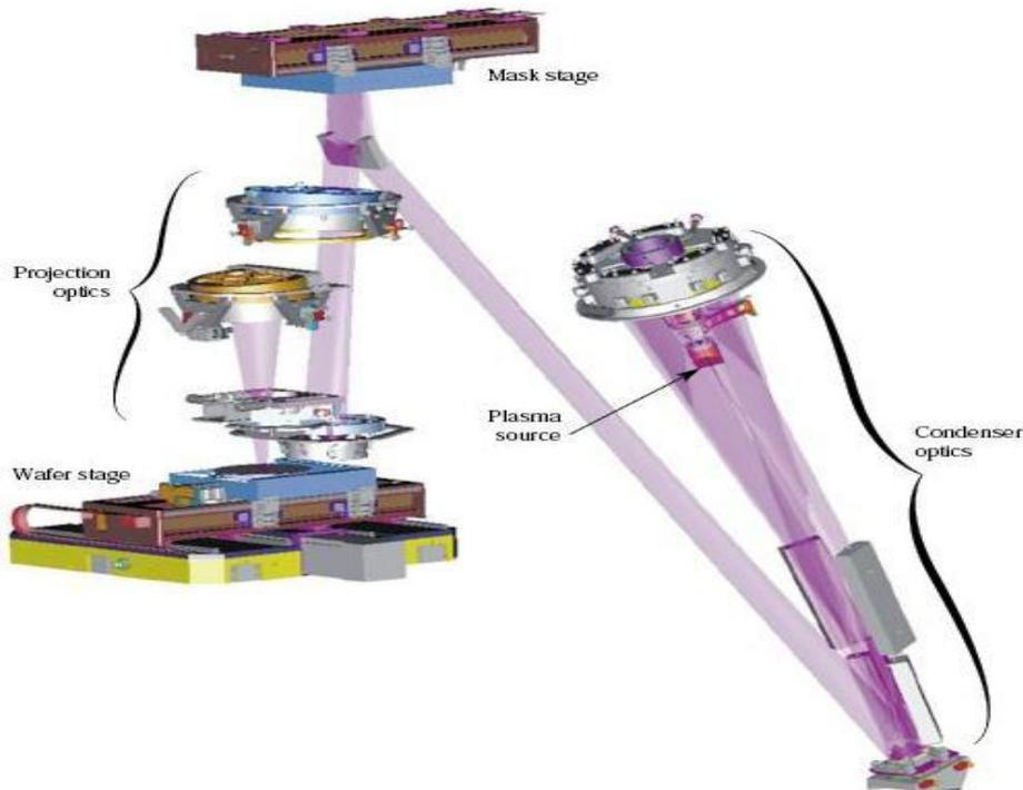
Fig-2: Basic diagram of the EUVL setup [5]
