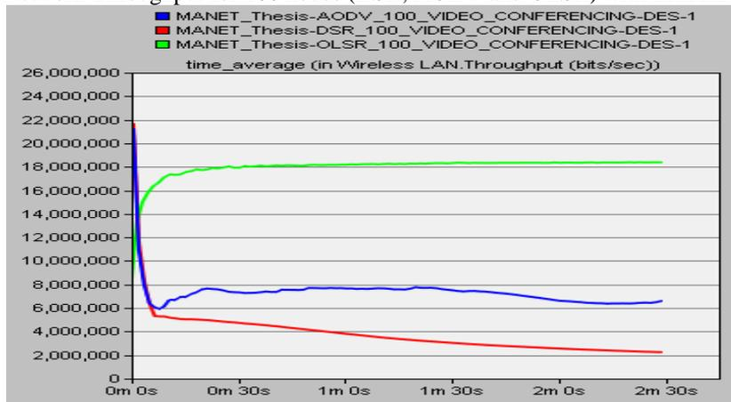
Fig. 9 Network Throughput for 100 nodes (DSR, AODV and OLSR) with VIDEO\_CONFERENCING Traffic.
