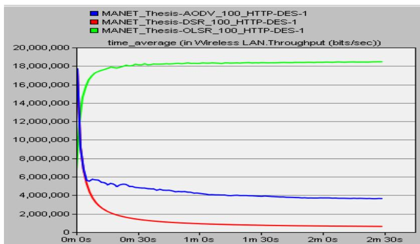
Fig. 7 Network Throughput for 100 nodes (DSR, AODV and OLSR) with HTTP Traffic.
