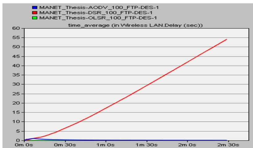
Fig. 10 Network Delay for 100 nodes (DSR, AODV and OLSR) with FTP Traffic.
