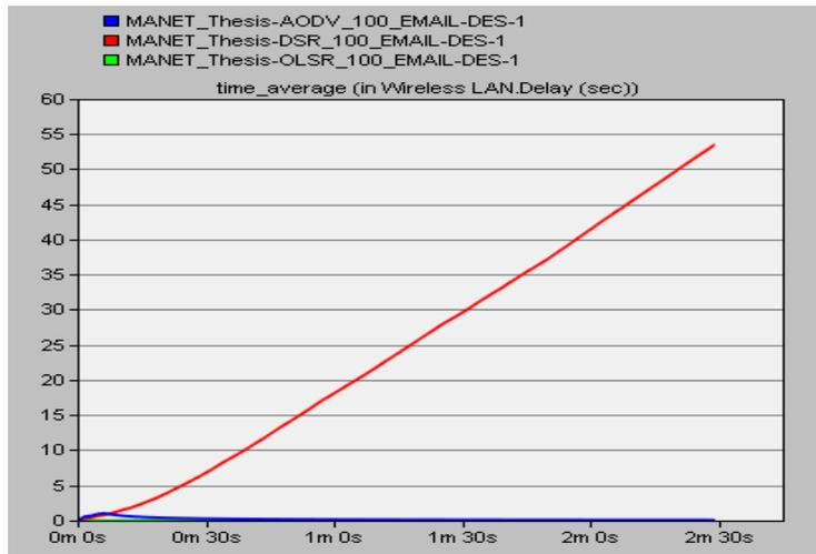
Fig.12 Network Delay for 100 nodes (DSR, AODV and OLSR) with EMAIL Traffic.
