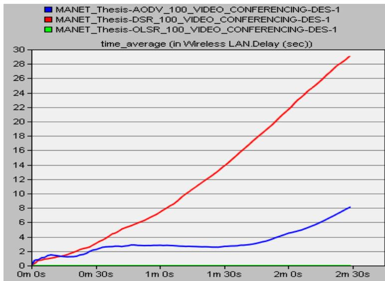
Fig.13 Network Delay for 100 nodes (DSR, AODV and OLSR) with VIDEO\_CONFERENCING Traffic.
