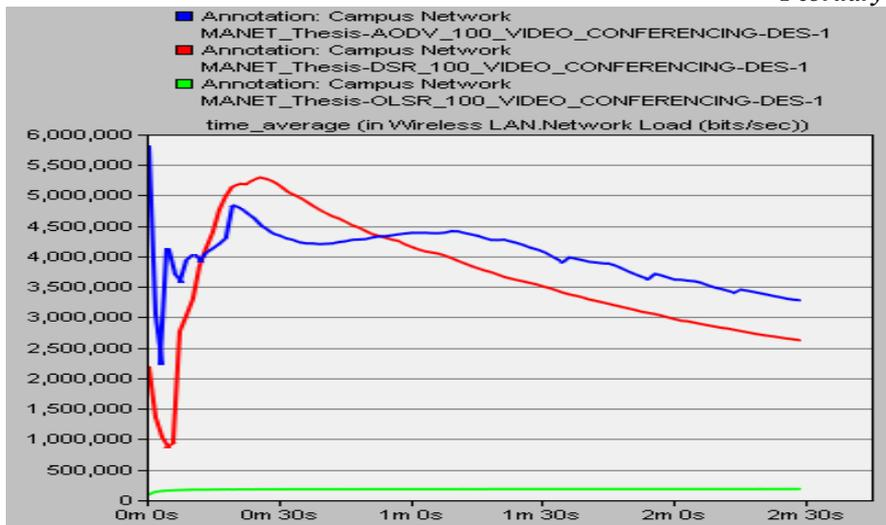
Fig. 5 Network Load for 100 nodes (DSR, AODV and OLSR) with VIDEO\_CONFERENCING Traffic
