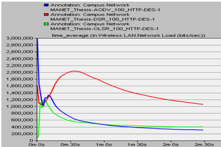
Fig. 3 Network Load for 100 nodes (DSR, AODV and OLSR) with HTTP Traffic.
