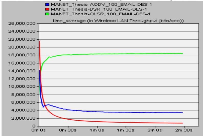
Fig. 8 Network Throughput for 100 nodes (DSR, AODV and OLSR) with EMAIL Traffic.
