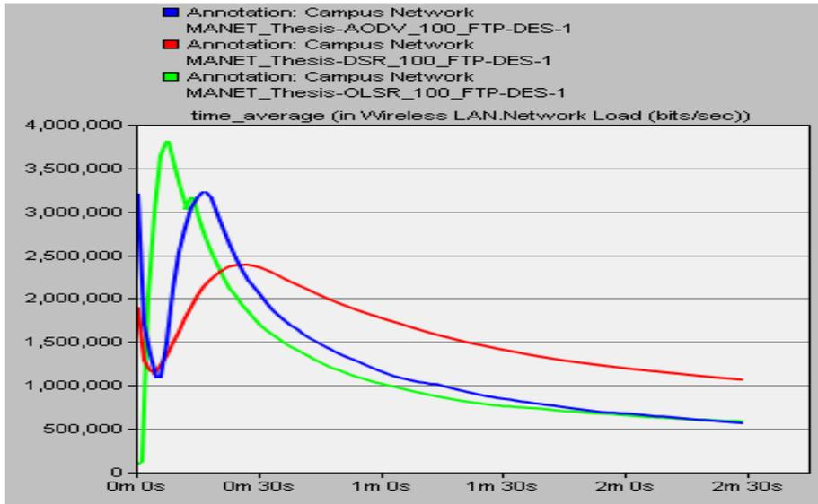
Fig. 2 Network Load for 100 nodes (DSR, AODV and OLSR) with FTP Traffic.
