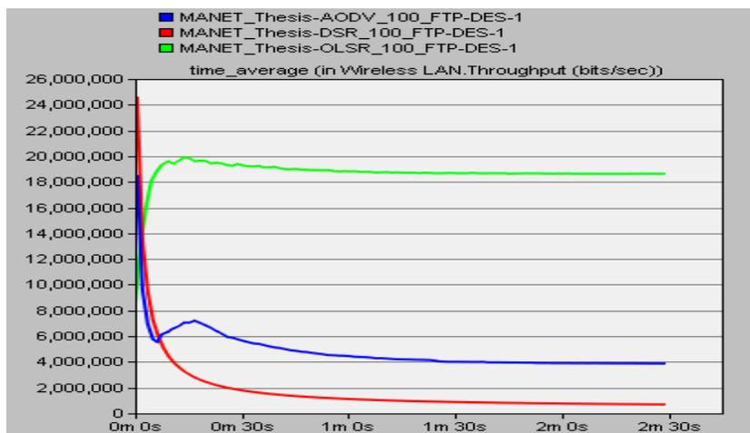
Fig. 6 Network Throughput for 100 nodes (DSR, AODV and OLSR) with FTP Traffic.
