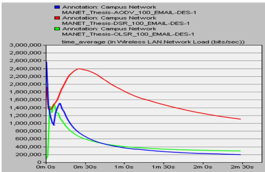
Fig. 4 Network Load for 100 nodes (DSR, AODV and OLSR) with EMAIL Traffic.
