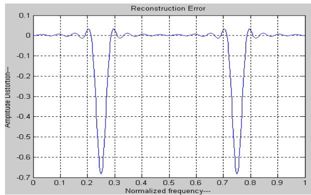
Figure 5: Variation of The Reconstruction error (kaiser window) by table 3. (previous work output using MATLAB))
