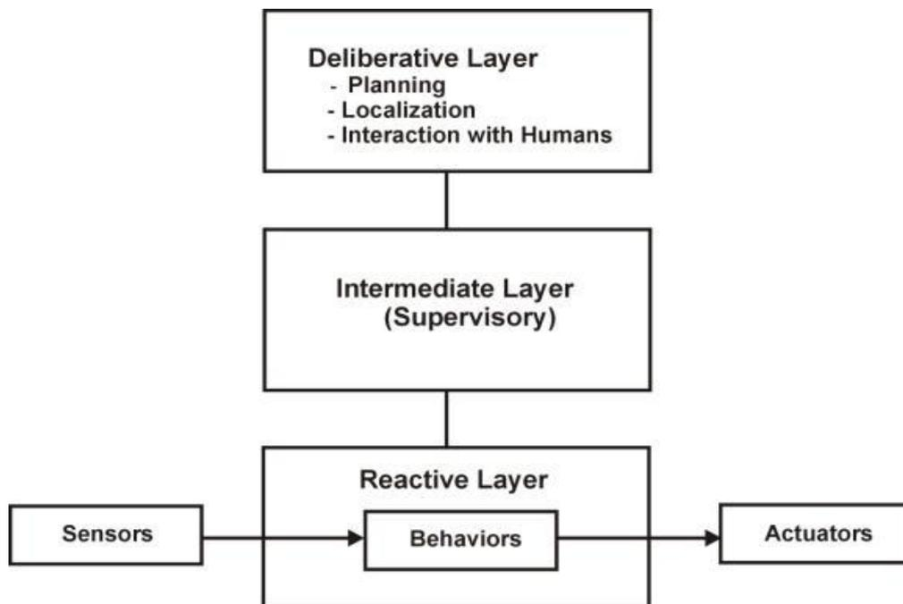
Fig 8.Three level Architecture for Robot Control
