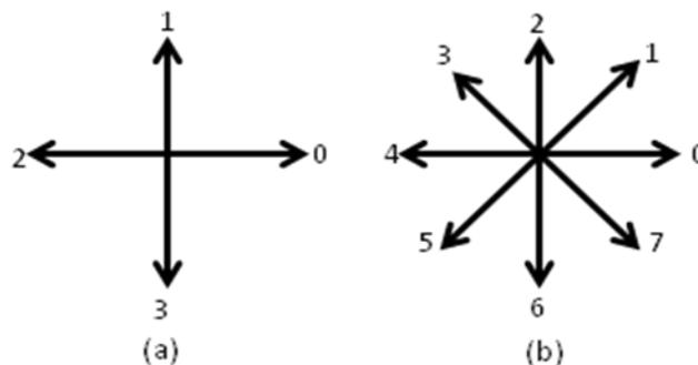
Fig. 2 Freeman Chain code using (a) 4- connectivity and (b) 8- connectivity
