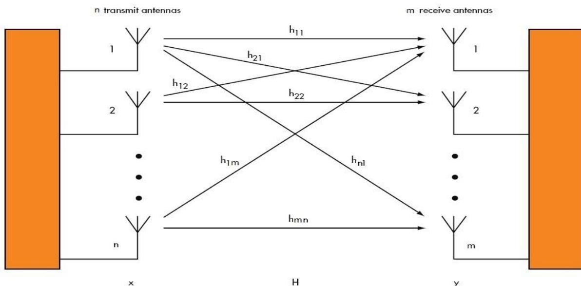
Fig. 4. A MIMO system consists of  $n$  transmit antennas and  $m$  receive antennas. Since the same channel is used, each antenna receives the direct component intended for it as well as the indirect components for the other antennas.
