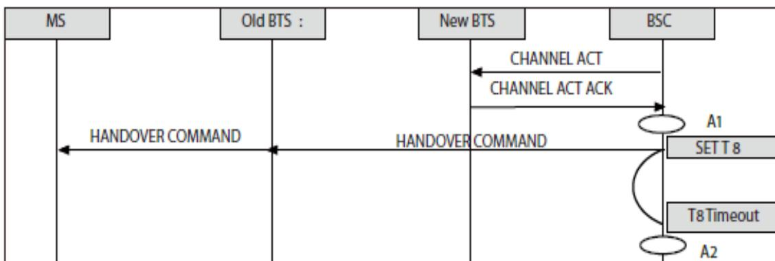
Figure 3. T8 Timeout (inter -cell handover failure under different BSC)
