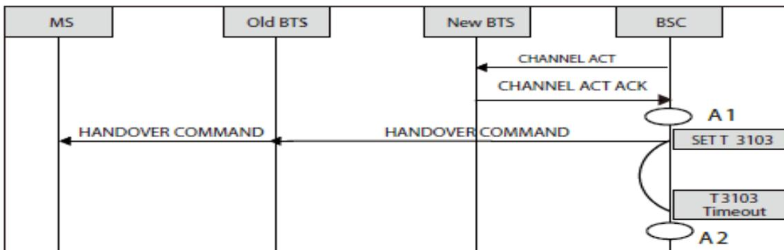
Figure 2. T3103 Timeout (inter -cell handover failure)
