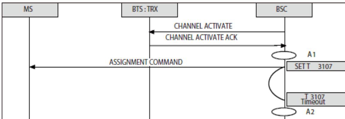
Figure 1. T3107 Timeout ( intra -cell handover failure)
