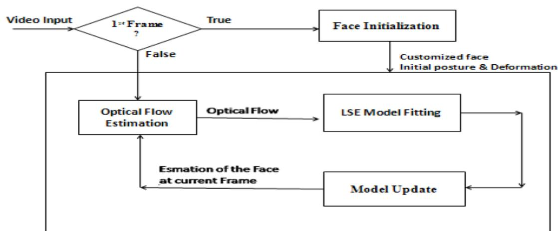
Figure 2: The flowchart of tracking procedure
