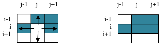
Figure 4.3. Filling gaps in a block image
