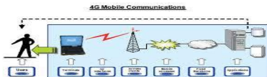
Fig 8 4G Mobile Communication System
