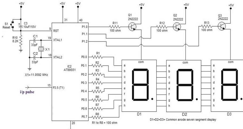
Fig 4: Heart rate monitor using 8051 microcontroller
