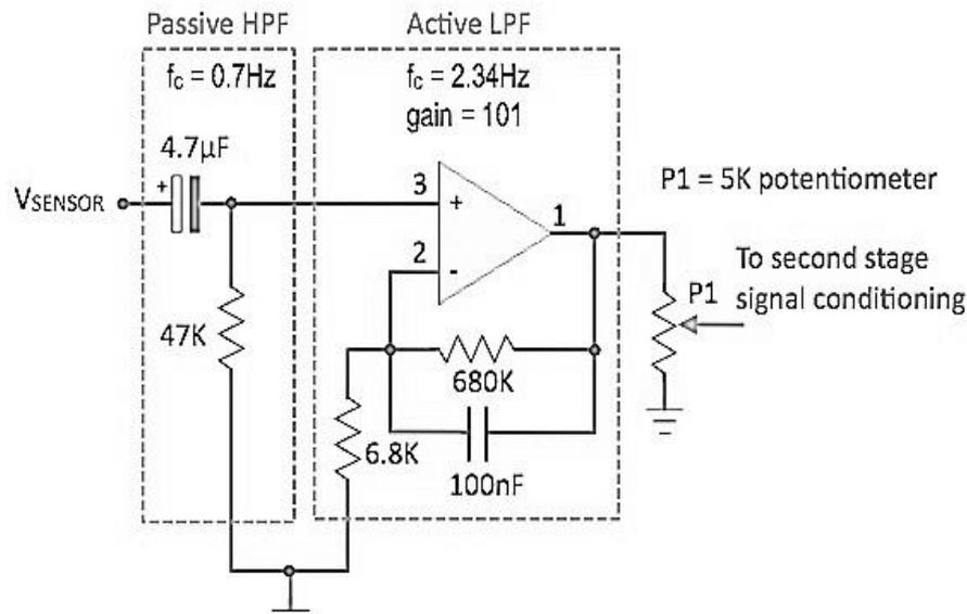
Fig 2: First Filter stage
