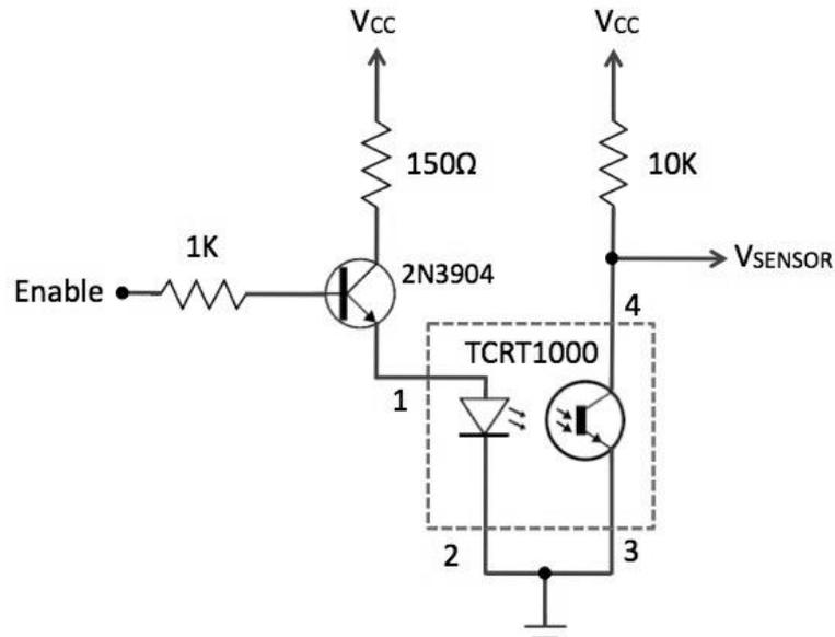
Fig 1: PPG sensor circuit
