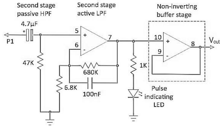
Fig 3: 2nd stage filtering
