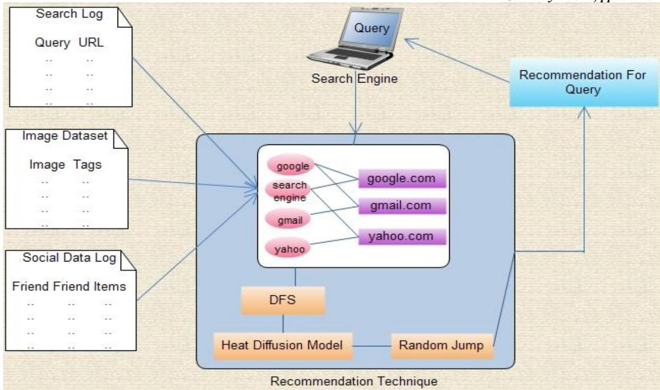
Fig.2 Web graph mining base recommender system Architecture
