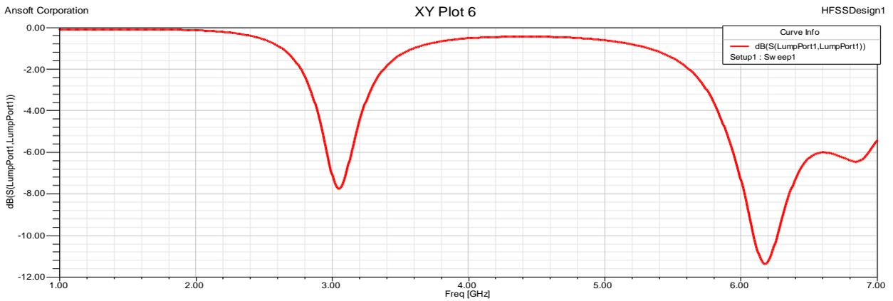
Figure 4: Simulated return loss [S11]
