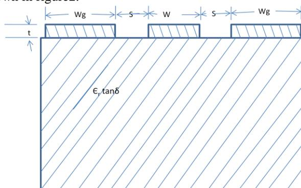
Figure: Cross sectional structure of coplanar waveguide
