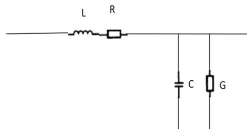
Figure2: Equivalent circuits of coplanar waveguide
