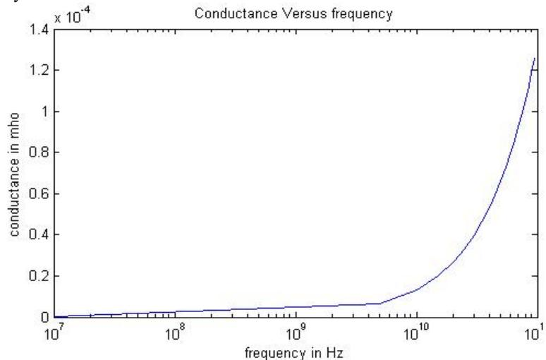
Figure5: Conductance versus frequency for coplanar waveguide
