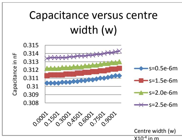
Figure3: Capacitance versus centre width of the coplanar waveguide with different slot width
