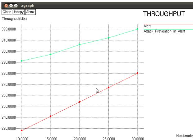
Figure Shows the throughput. In the X-axis number of nodes is taken. In Y-axis throughput is taken. In the existing system, Anonymous Location-based Efficient Routing protocol is used. The proposed system has to detect and prevent black hole and Flooding attacks. When compared to the existing method, there is high throughput in the proposed system.
