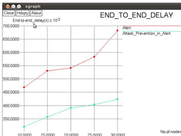
Figure Shows the end-to-end delay. In the X-axis number of nodes is taken. In Y-axis packet delivery ratio is taken. In the existing system, Anonymous Location-based Efficient Routing protocol is used. The proposed system has to detect and prevent black hole and Flooding attacks. When compared to the existing method, there is less end-to-end delay in the proposed system.
