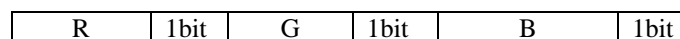
Fig.03 One RGB pixel to store three secret data bits. One bit per each rgb pixel.
