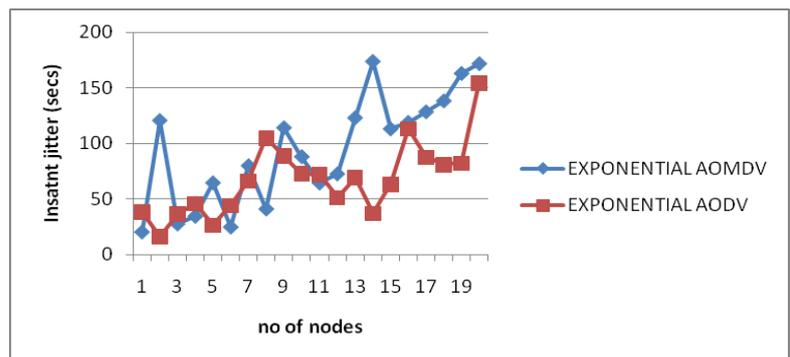
Fig 11. Instant jitter versus no of nodes (Exponential)
