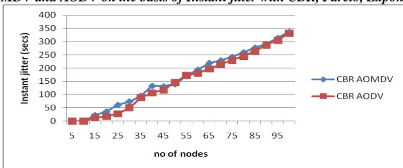
Fig 9. Instant jitter versus no of nodes (CBR)
