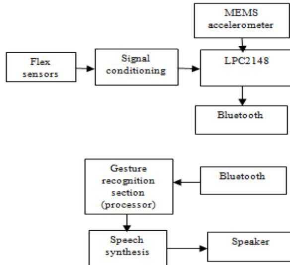
Fig 1 Block diagram of hand gesture recognition
