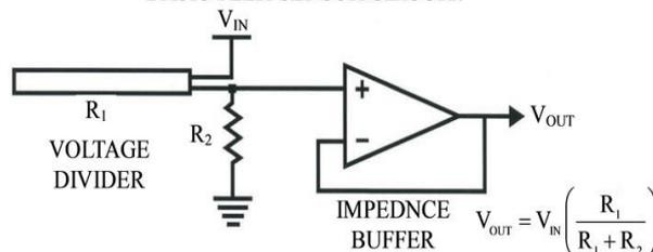
Fig 3. Basic flex circuit diagram
