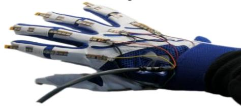
Fig 2 Data glove with flex sensors.
