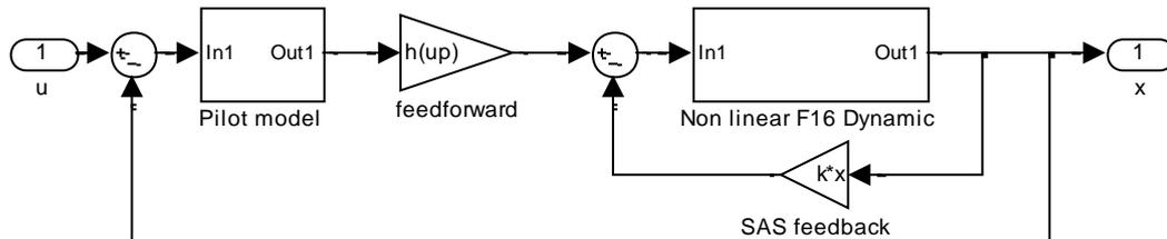
Fig. 8 Pilot-aircraft in the loop
