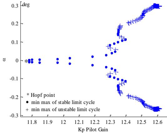
Fig. 10 Stable and unstable limit cycles for  $\tau = .15$  as Kp varies
