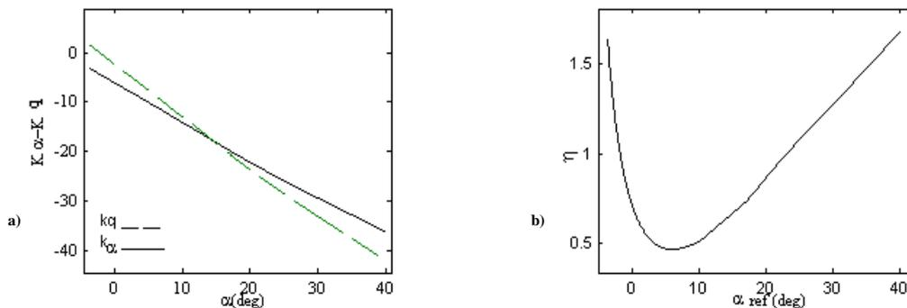
Fig. 1 a) Quasi-linear attack angle and pitch rate feedback gains b) feed-forward trust correction
