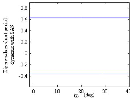
Fig. 4 : New poles position for Short Period F16 dynamic with the designed SAS
