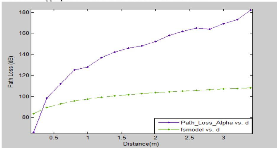
Figure1: Comparison of measured with free space path loss model
