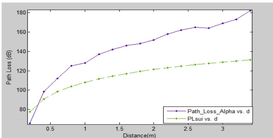
Figure3: Comparison of measured with free SUI model
