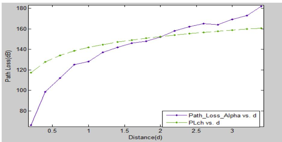
Figure2: Comparison of measured path loss with theoretical COST-Hata model
