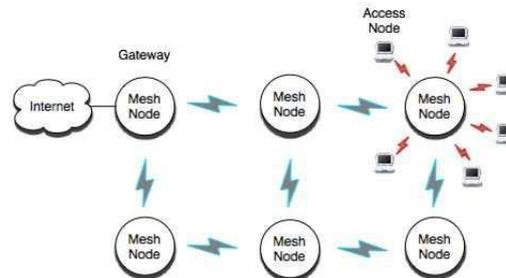
Fig 2 A two-tier networks consist of infrastructure nodes which forward packets and client nodes which only originate or source traffic.
