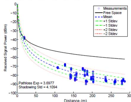
Fig 3 Empirical data and theoretical predictions for signal power received from an access node at 1 meter with a low gain antenna from a transmitter at 10 meters having a 15 dBi antenna.
