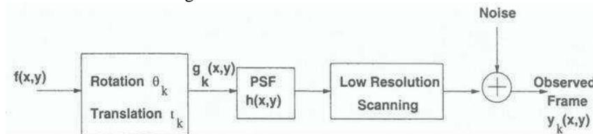
Figure 1 Observation Model relating a High Resolution Image to Low Resolution Frames.
