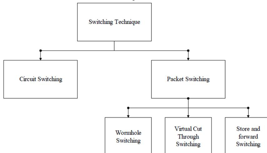
Figure 1.2 Switching Techniques in NoC
