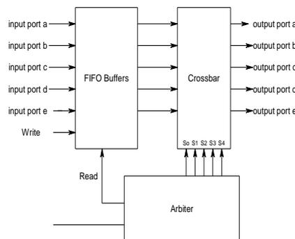
Fig. Block Diagram NoC Router
