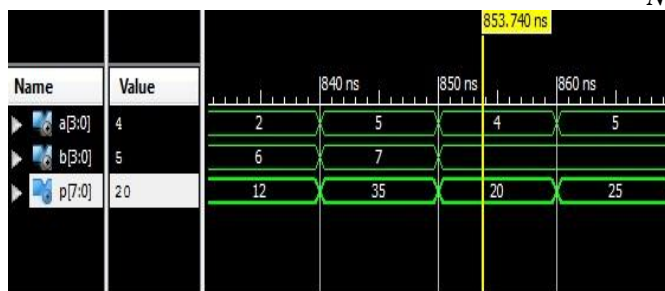
Fig-6: Simulation waveform of Proposed 4x4 Vedic multiplier
