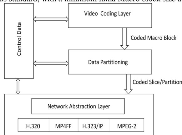
Figure 2. Structure of H.264/AVC Video Encoder
