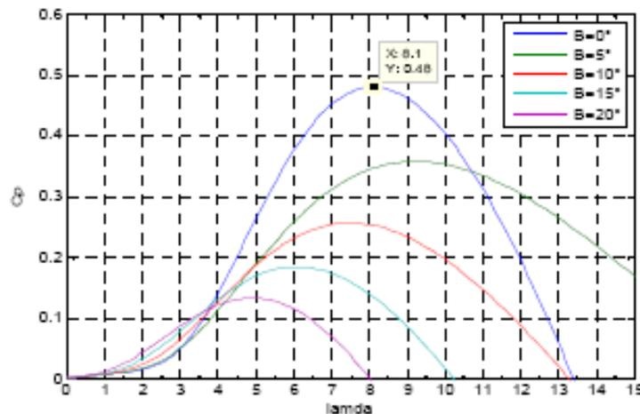
Figure 2: Aerodynamic Power Coefficient Variation  $C_p$  against Tip Speed Ratio  $\lambda$  and Pitch Angle  $\beta$
