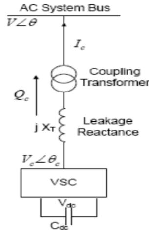
Figure 3: The schematic diagram of STATCOM
