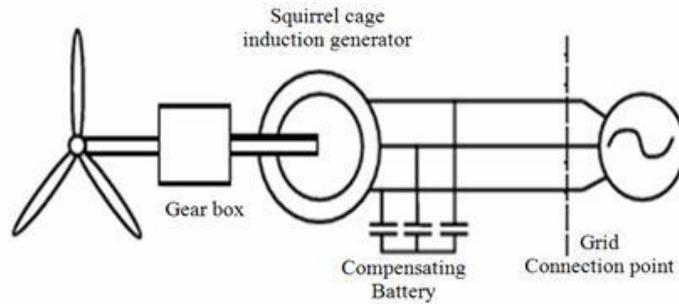
Figure 1 : Squirrel cage induction generator
