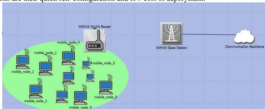
Fig.1 MANET deployment over WiMAX
