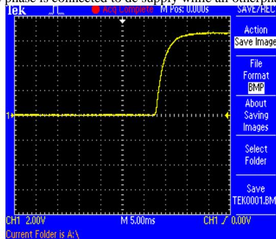
Fig 7: Current through the Motor Phase Winding
