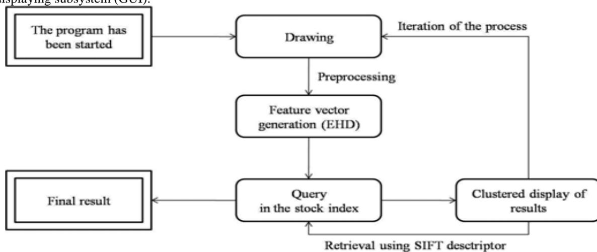
Fig: The data flow model of the system from the user's point of view.
