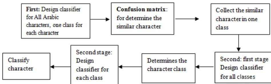
Figure 4. A new proposed approach with two stages of classifiers
