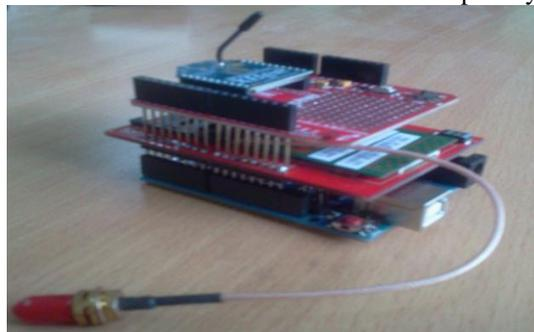
Fig. 2 Sensor Gateway Hardware
