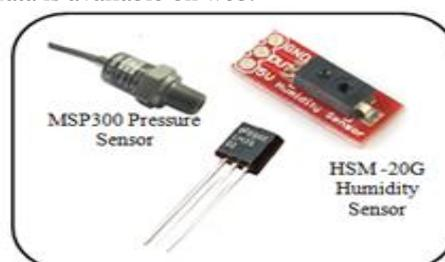
Fig. 3 Sensors Connected to Microcontroller Board
