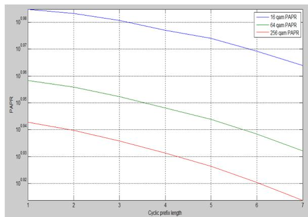
Fig.4. PAPR reduction curve representation by reducing length of cyclic prefix using 16, 64 and 256 QAM modulation techniques.
