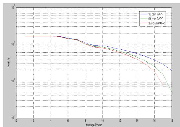
Fig.5. PAPR reduction curve representation of OFDM system by increasing the average power of signal using different modulation techniques.
