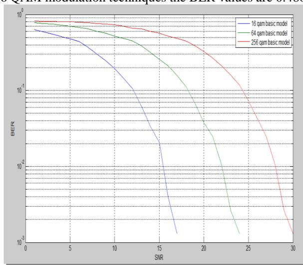
Fig.1. BER curve simulation of basic OFDM model using 16, 64 and 256 QAM technique over an AWGN channel.
