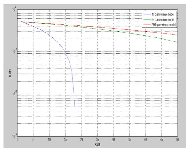
Fig.2. BER curve simulation of OFDM based Wimax model using 16, 64 and 256 QAM technique over an AWGN channel.
