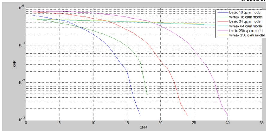
Fig.3. BER curve comparison of Basic and Wimax model using different modulation techniques over AWGN channel.
