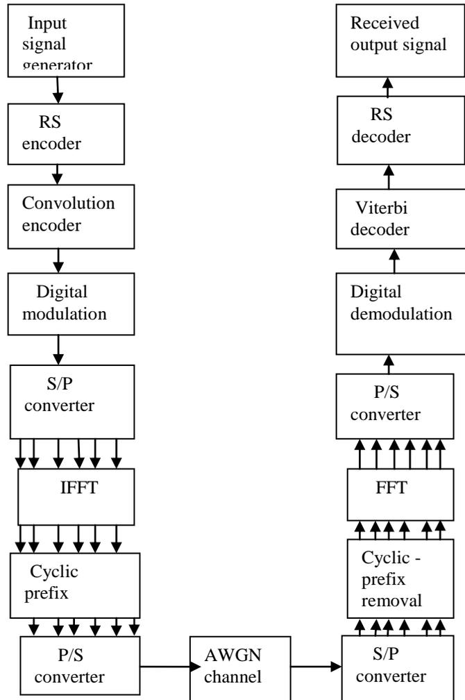
Fig. b. OFDM based Wimax Physical layer transceiver model
